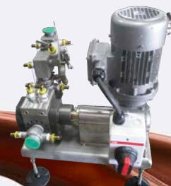
CHOCOLATE LOBE PUMP TO CONTINUOUSLY FEED THE ENROBER
